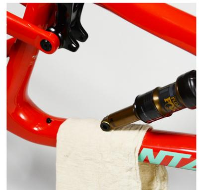
6. Rotate the frame to expose the grease port of the lower link.
