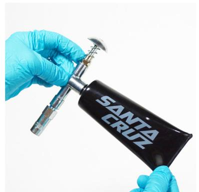
4. Squeeze the grease gun into a rag until you see a consistent flow of grease.
