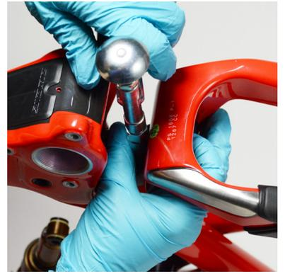
10. Use a 6 mm hex wrench to reinstall the shock bolt and torque to 15.8 N·m (140 in-lb).
