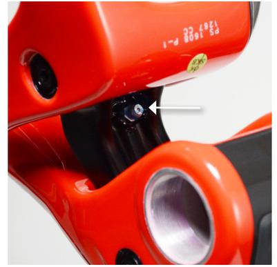
7. With the knurled end loose, firmly press the grease gun onto the lower link fitting. Hand-tighten the knurled cap to secure the grease gun.
