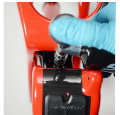
9. Unscrew the knurled cap and remove the grease gun from the fitting.
