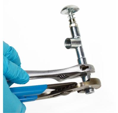
2. Turn the knurled cap counter-clockwise by hand until it stops.
