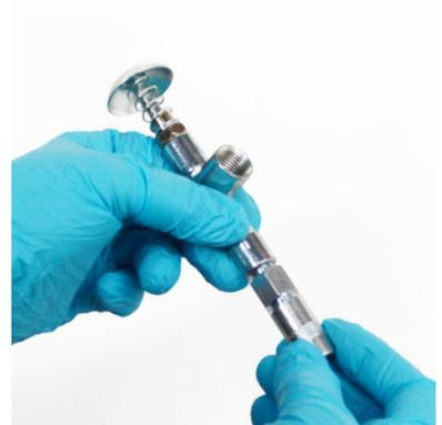
3. Thread the container of Santa Cruz grease onto the grease gun.
